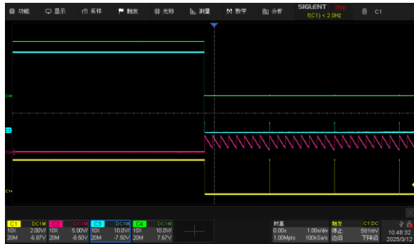
Over current protection
