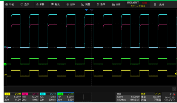
Continues repeated switch on an off with 3A load
