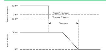
Gate Shut Down Timing in the Event of Reverse Polarity VCAPH and VCAPL Pins
