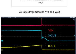
Input over voltage protection release
