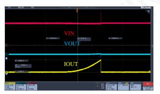
Output short circuit protection in startup
