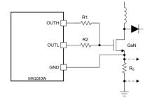
To prevent this, a common-mode choke can be used for IN+ and IN-, respectively. Resistors can also add to the signal output line before MX1020W depending on the input signal pulse width to provide additional RC filtering as shown in the following figure.
