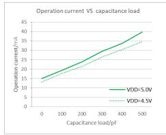
Operation current with different capacitance load
