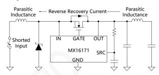
Reverse Recovery Current Generates Inductive Spikes at  $V_{\rm IN}$  and  $V_{\rm OUT}$  pins
