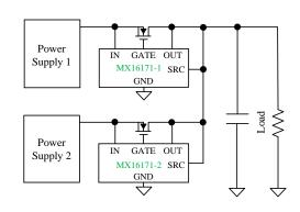
Typical Redundant Power Supply Configuration
