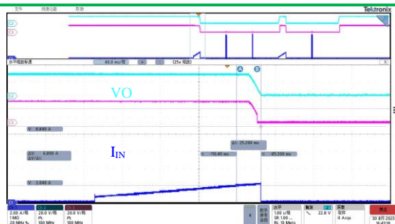
Overload Performance with MX26631S during Load Step from 0A to 3A
